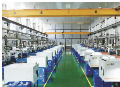
CNC Horizontal Injection Molding Machine
